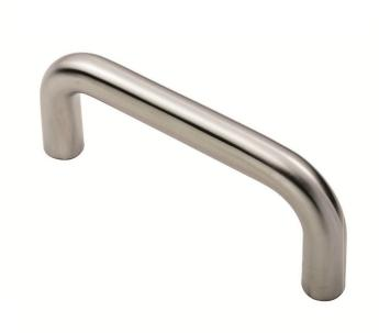
A robust and functional 19mm Dia. round bar D type pull handle, part of the Steelworx range in grade304 Stainless Steel, so ideal for internal and external homes and offices. Available in different sizes. These pull handles are fixed with 2no M8 threaded bolts through the door giving the strongest fixing possible.
