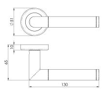
Lever on a concealed fix 2 part screw on round rose. The Trend lever is a round bar sectional lever with a mitred corner. A favoured choice within the Serozzetta range, the timeless design is guaranteed to suit both the home and office environment. The chamfered edge concealed fix rose reflects the attention to detail in this range.
