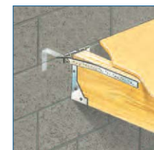
Floor level straps. 150 x 650mm long once bent and once twisted fixed to perpendicular joists.
