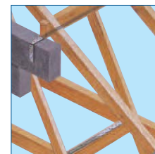
Anchorage of gable end to roof structure.
