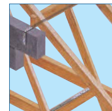
Anchorage of gable end to roof structure.
